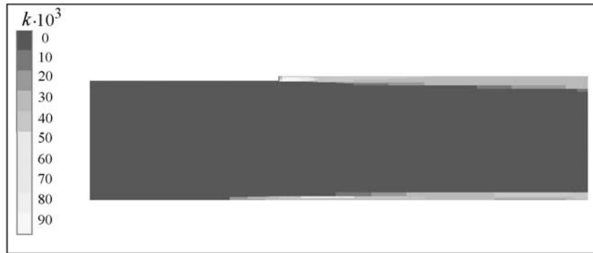
Fig. 13. Distribution of the turbulent kinetic energy k \cdot 10^3 \text{ m}^2/\text{s}^2 in the model of the channel. k, \text{ m}^2/\text{s}^2 .
